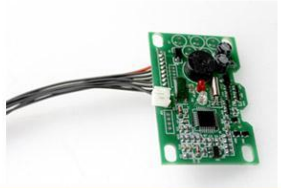
Pcb board:no Independent clock chip MF chip often loss information
