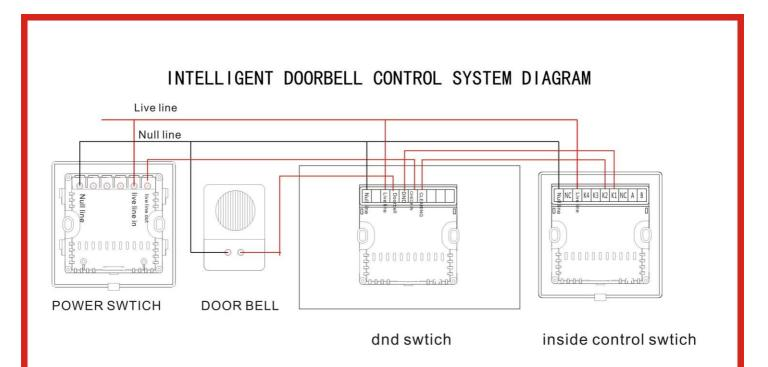
Remarks: All of the wire should apply powerline, diameter of which equals 0.5 square meter or more.
